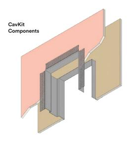
CavKit is a trim kit only and does not include the cavity sliding door, frame or track. CavKit is designed to suit most brands of cavity sliders. CavKit standard components assumes the lining board is the same on both sides. Please contact Studco if the lining boards are not equal thickness.
